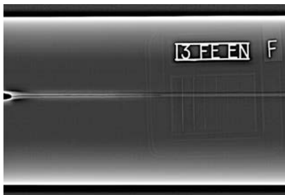
Thin-walled stainless steel cylinder with longitudinal weld seam.
